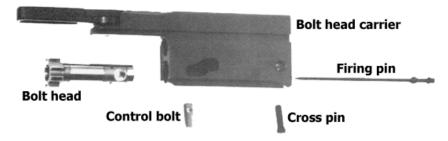
Fig. 41: Bolt, disassembled
