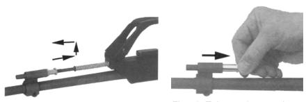
Fig. 39: Remove the push rod
