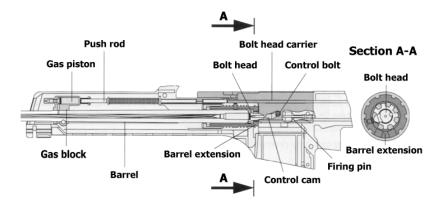
Fig. 31: Bolt, locked
