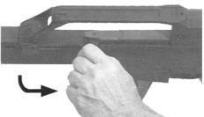
Fig. 33: Swivel out and pull back cocking lever
