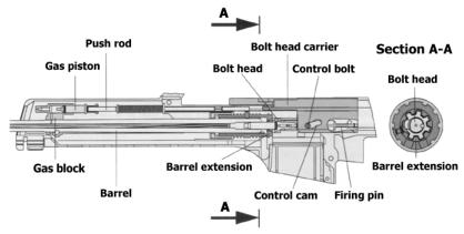
Fig. 32: Bolt, unlocked
