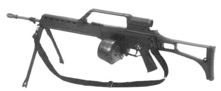
Fig. 5: MG36 E with drum-type magazine, bipod and carrying sling, left side view
