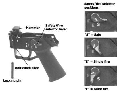
Fig. 14: Pistol grip with trigger mechanism
