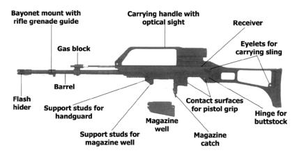
Fig. 8: Receiver with barrel, buttstock and attaching parts.
