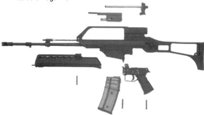
Fig. 45: G36 E disassembled into assembly groups.
