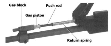
Fig.9: Gas operation assembly
